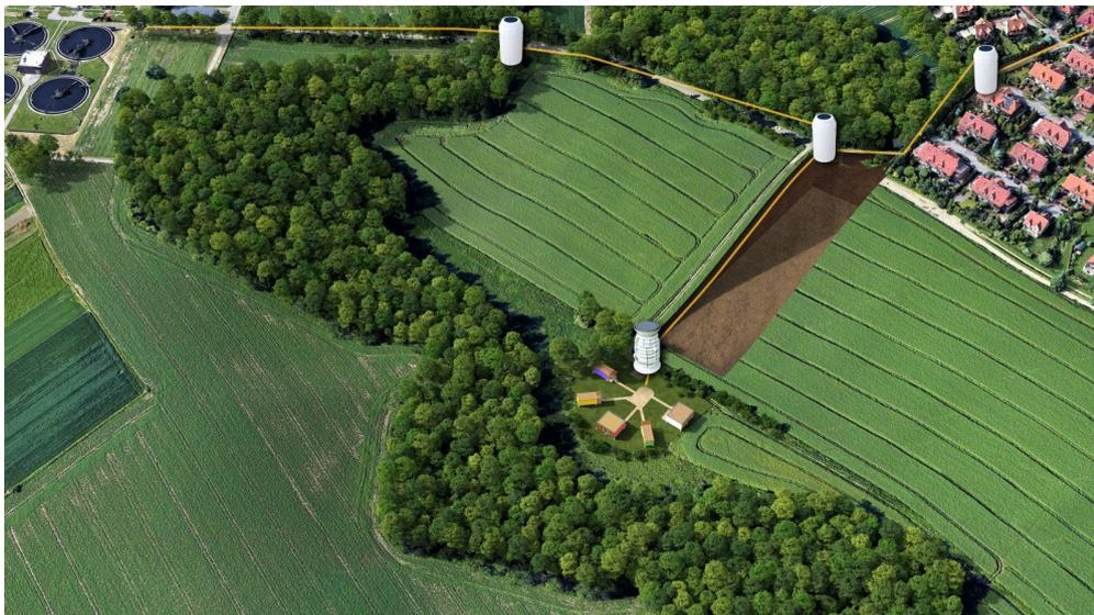
*Fig 2: A Tiny House settlement connected to the public sewer system via a pressure drainage system, allowing wastewater to be properly treated. (Picture: Jung Pumpen)*
