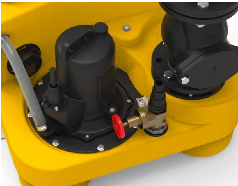
Pic 3) Compli 400: With the emergency disposal connection, available as an accessory, the tank can be emptied by means of a wet vacuum cleaner or hand diaphragm pump if necessary.
